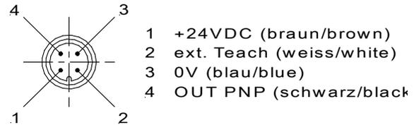
View to the connector on the sensor
